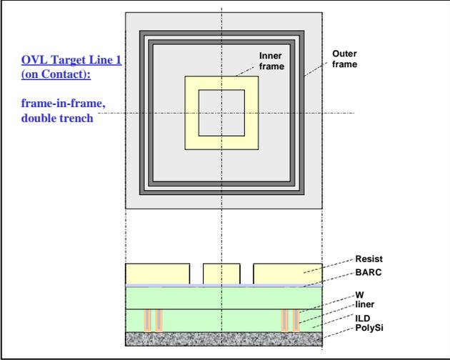
**Figure 1a:** line 1 overlay target design
