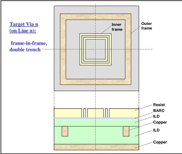
**Figure 1c:** via n on line n target structure
