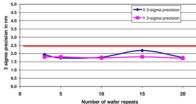
**Figure 2:** impact of the number of measurement repeats on 3-sigma precision
