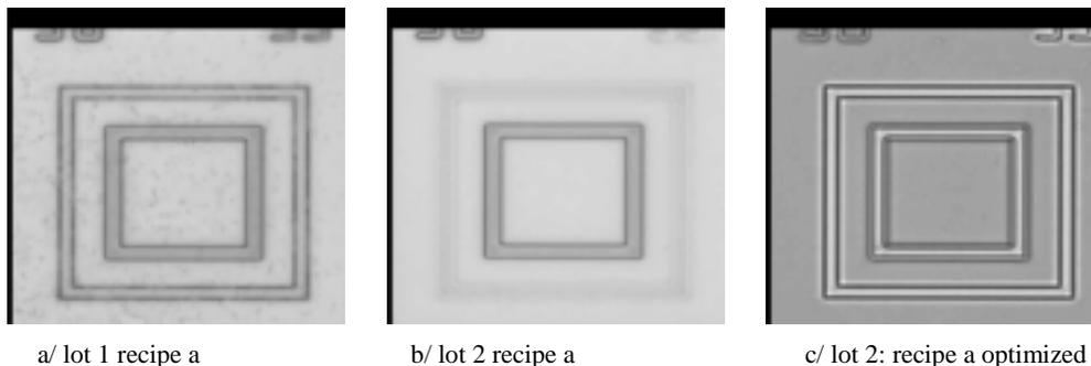
**Figure 4:** Line 4 overlay targets for two production lots 1 & 2. Pictures a & b describe contrast variations observed between lots 1 & 2. Picture c describes contrast enhancement obtained after recipe optimization.
